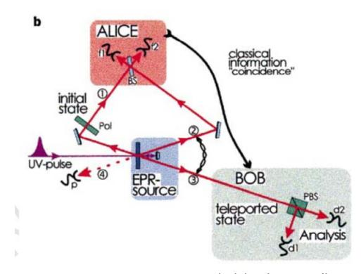
polarizing beam splitters (PBS) as detectors of teleported states
