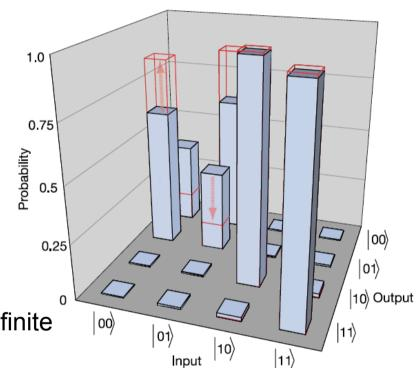
Deviation from expected accuracy due to finite rise/fall time of pulse
