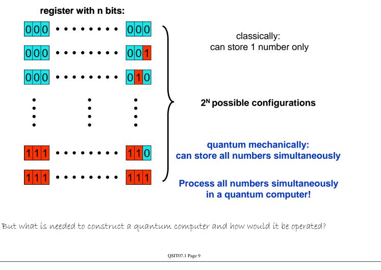
Schematic of a Generic Quantum Processor
