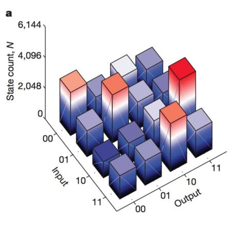
error sources: decoherence, control errors and 40% measurement visibility
