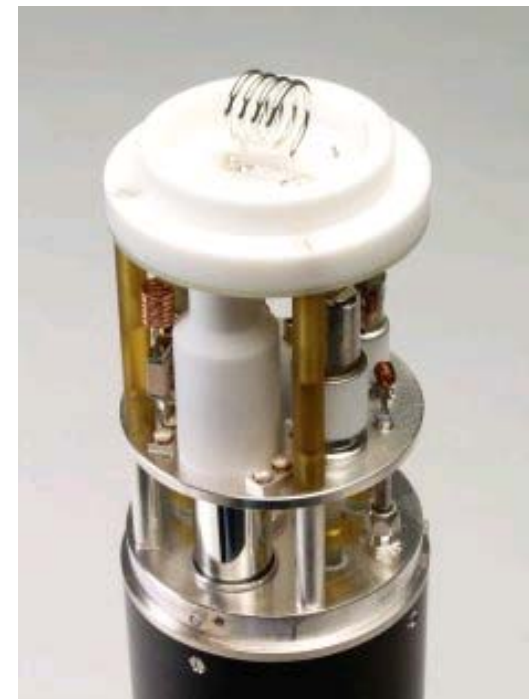
Transmission / Receiver coil
