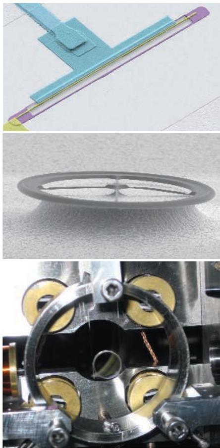
**Many sizes.** Physicist are experimenting with nanometer-sized beams (top), micrometer-sized rings (middle), and macroscopic mirrors.
