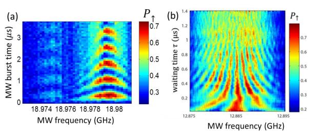
Fig. (a) Measured spin-up probability as a function of MW frequency and burst time. (b) Measured spin-up probability as a function of MW frequency and waiting time  $\tau$  between two  $\pi/2$  (75 ns) pulses with equal phase, showing Ramsey interference.
