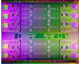
3.000.000.000 transistors smallest feature size 32 nm clock speed ~ 3 GHz power consumption 10 W
