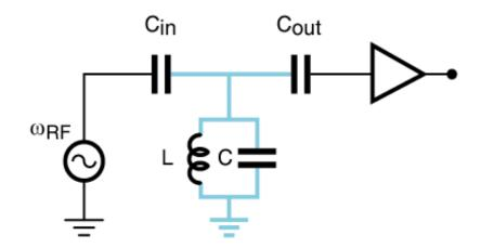
photon lifetime (quality factor) controlled by coupling capacitor C<sub>in/out</sub>
