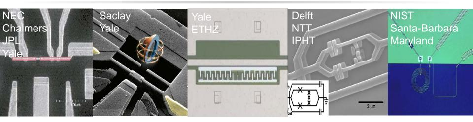
'artificial atoms' -- single superconducting qubits
