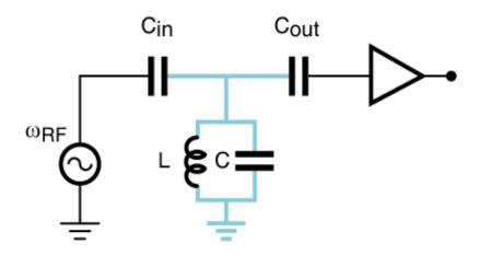
photon lifetime (quality factor) controlled by coupling capacitors  $C_{in/out}$
