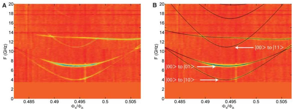
fitting are  $I_{p1}/h = 873 \pm 13$  GHz/ $\Phi_0$ ,  $I_{p2}/h = 705 \pm 19$  GHz/ $\Phi_0$ ,  $I_{p3}/h = 516 \pm 35$  GHz/ $\Phi_0$ ,  $\Delta_1/h = 4.022 \pm 0.078$  GHz,  $\Delta_2/h = 6.915 \pm 0.075$  GHz,  $\Delta_3/h = 12.454 \pm 0.074$  GHz,  $\Delta\Phi_1 = 5.58 \pm 0.11$  m $\Phi_0$ ,  $\Delta\Phi_2 = 5.31 \pm 0.22$  m $\Phi_0$ ,  $J_{12}/h = -0.003 \pm 0.066$  GHz,  $J_{13}/h = 0.715 \pm 0.130$  GHz, and  $J_{23}/h = 0.482 \pm 0.171$  GHz.
