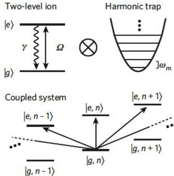
**Laser on carrier transition: manipulation of the internal state**
