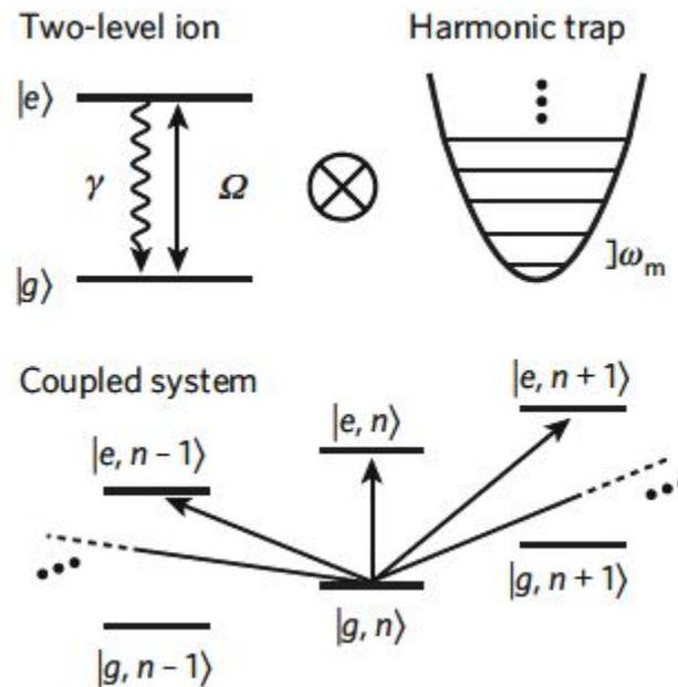
Energy levels of a two-level trapped ion
