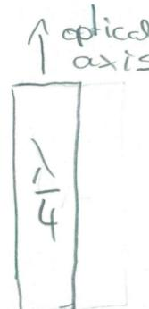
induces phase shift of  $\pi/2$  between e and o beams. turns linear into circular polarization at  $\pi/4$  incidence to optical axis
