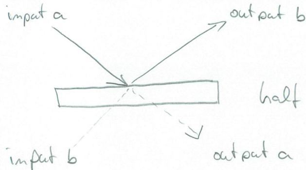
half silvered mirror = beam splitter (polarization independent)
