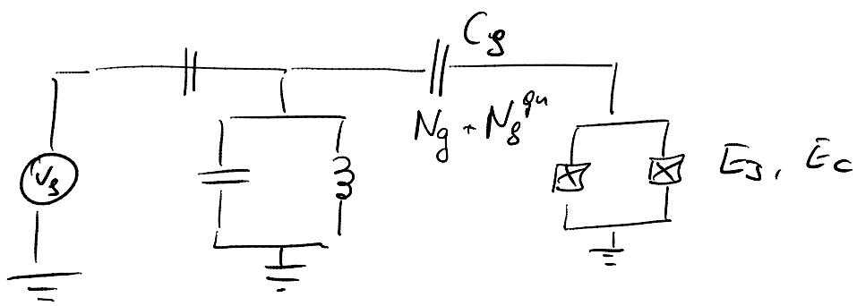
$N_g$  - polarization charge on  $C_g$
