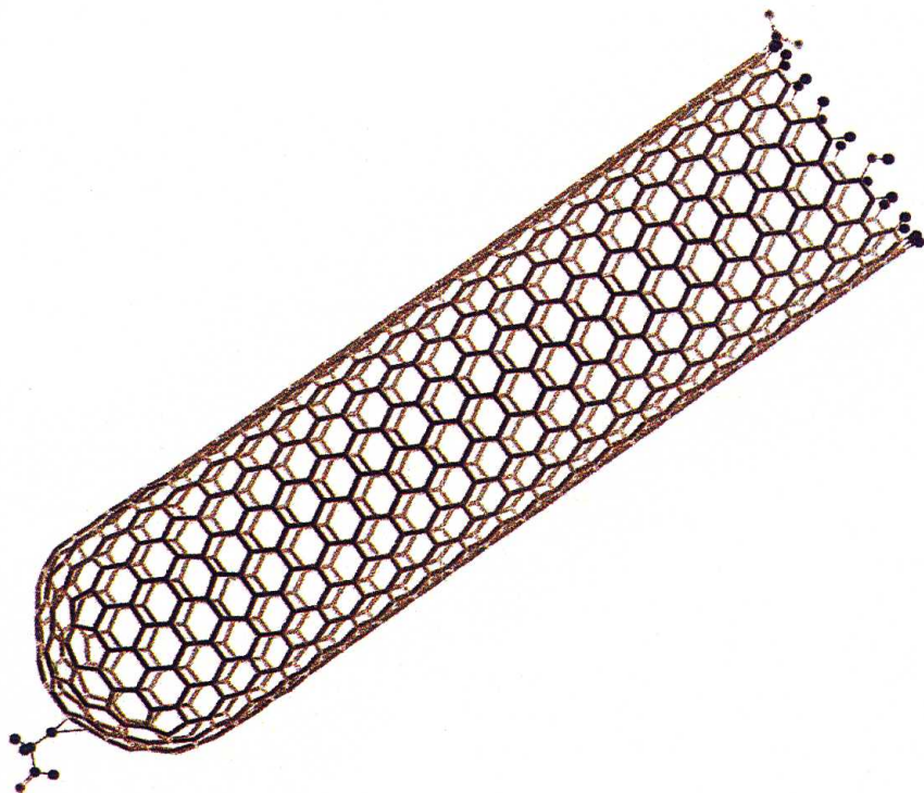
Figure 3. Derivitized section of a (10,10) fullerene nanotube with one end open.
